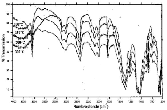
Figure 1. Infrared spectra of Na/FAP catalysts calcined at different temperatures.
