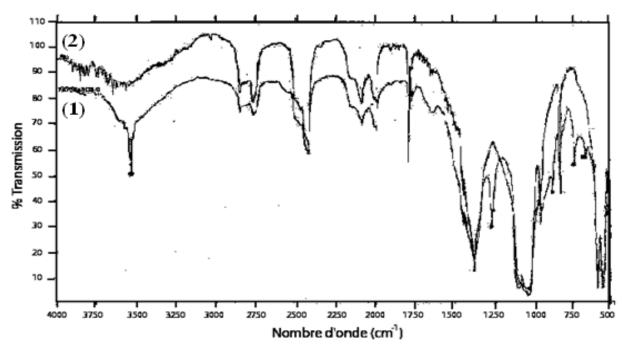
Figure 2. Infrared spectra of Na/FAP catalysts calcined (1) and no calcined (2).
